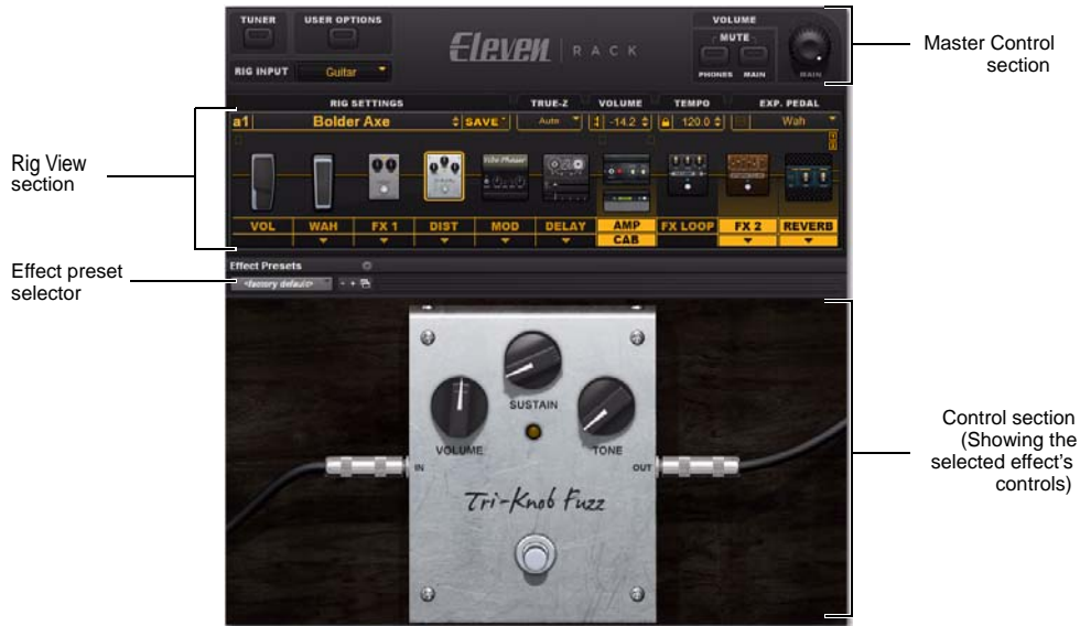
Figure 10. Eleven Rack Control window (in Pro Tools)
