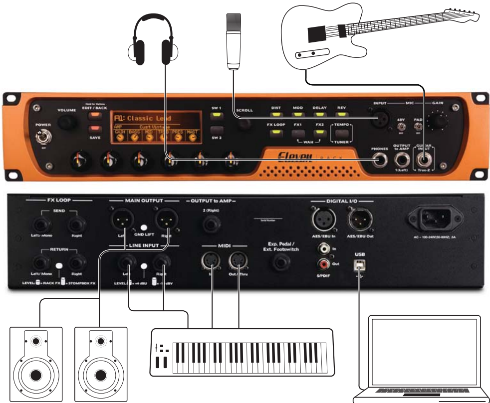
Figure 8. Studio Setup with Eleven Rack as your Pro Tools audio interface
