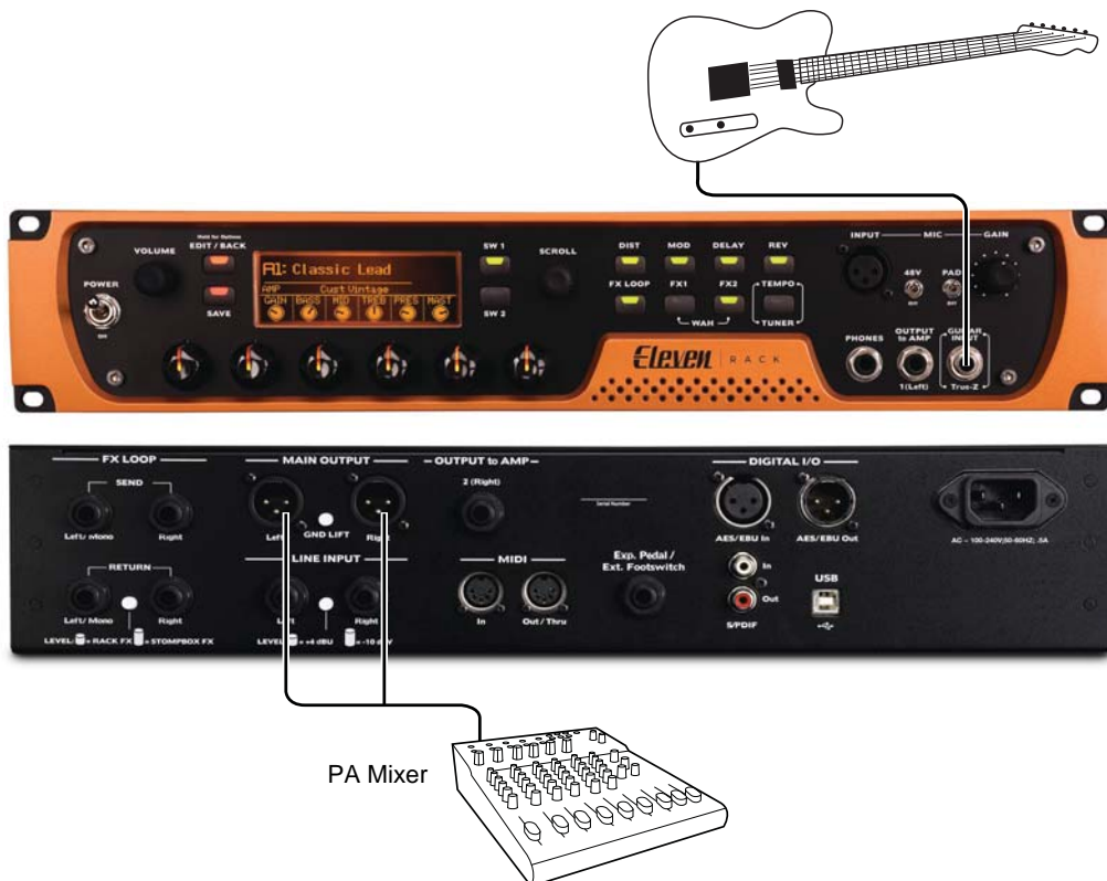
Figure 5. Eleven Rack connected directly to the PA mixer
