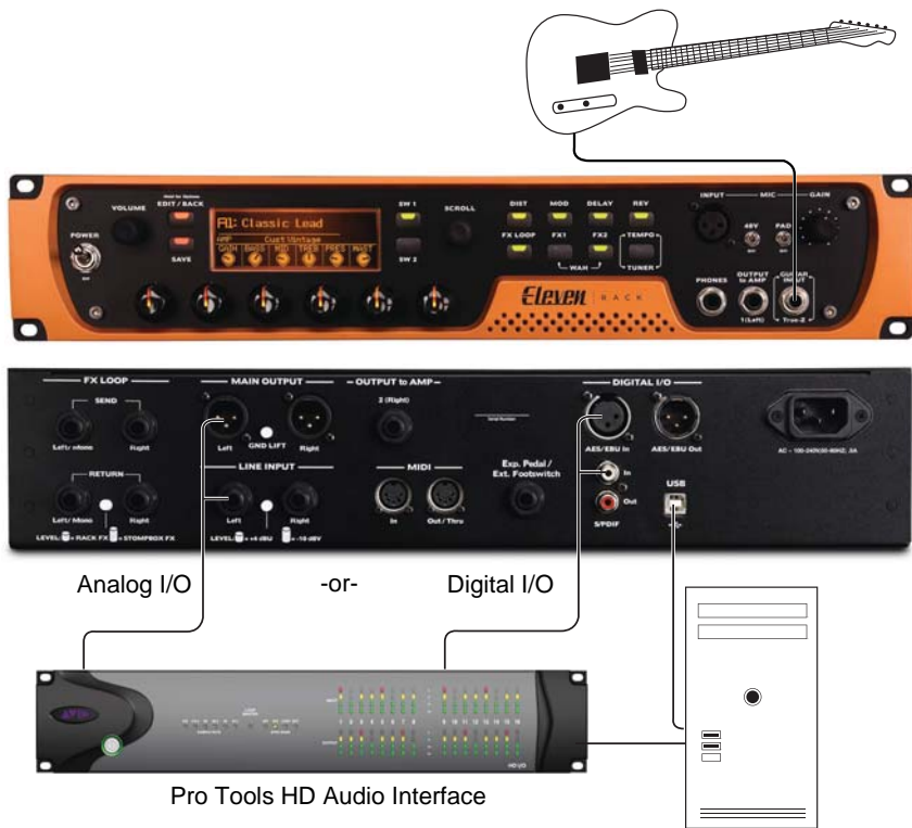
Figure 9. Eleven Rack connected to a Pro Tools|HD system
